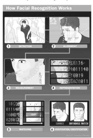
Fig. 1 the steps of 3D face recognition system.
